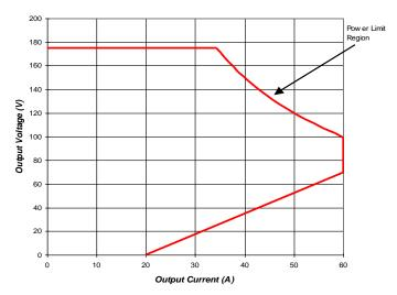
\*60A current limit automatically reduces by 0.6A/°C for heatsink temperatures above 60°C.
