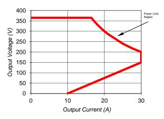
\*30A current limit automatically reduces by 0.3A/°C for heatsink temperatures above 60°C. \*maximum output 355VDC at 400VAC, 365VDC available at 415VAC and above.
