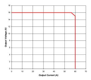
(1) During battery recharge the current limit reduces maximum power available
